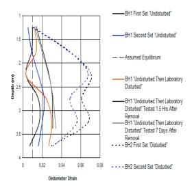
Some were tested in their undisturbed state, 1.5 hours following removal from the sample tube. Others were 'laboratory disturbed' and a third set were allowed to stand for several days prior to testing.
