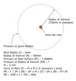
Clive Bennett provides the above area method of estimating pressure at any distance from the root by entering the suction exerted by the root, its radius and the distance to the point of interest.
